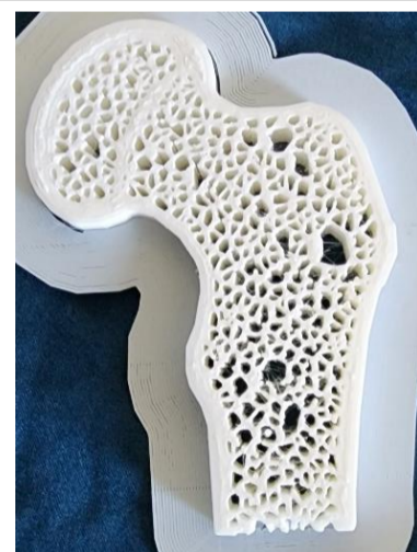
Figure 2: 3D Printed Bone with similar porosity (infill geometry) used in our studies
